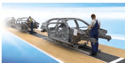
The Skid Transfer System
